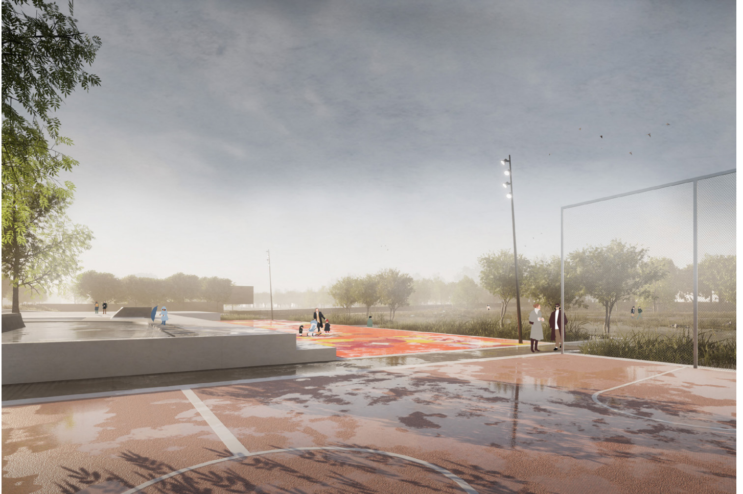
In times of bad weather, functions like the skatepark serve as a retention basin.
